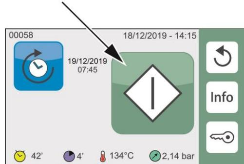
To this end, place the test device on the central tray without inserting other material. Close the door and start the cycle.
