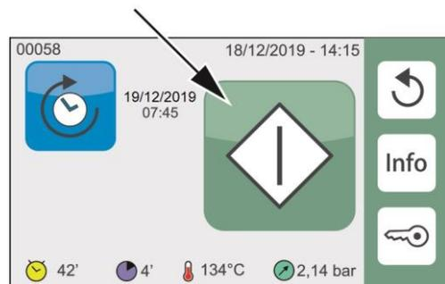
The cycle must run with the sterilisation chamber empty, and only the trays and their supports inserted.
