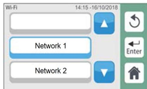
Following the selection of the network name, enter the network PASSWORD and confirm by pressing ENTER. SHIFT button allows special characters keyboard.
