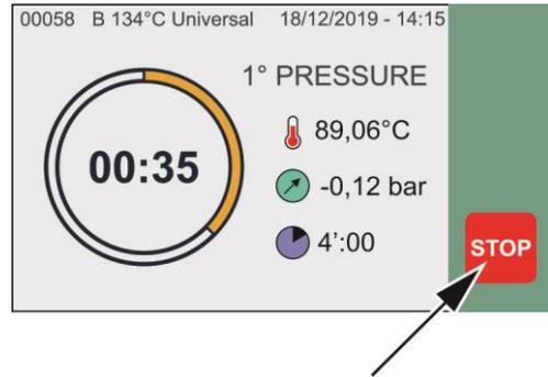
The command generates **E999 error** since the cycle could not finish correctly. Press ENTER to proceed.
