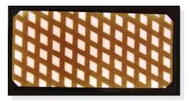
**PASS** Excessive dry time. Shorten dry time to 5 minutes or less for Bowie-Dick Test.
