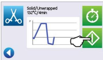
**7** When cycle is complete, press STOP, open door and remove load.
