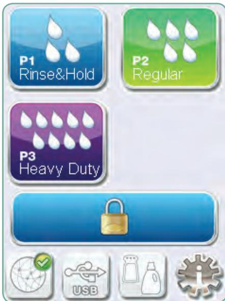
A high-resolution, 65K color touch screen offers a vivid display of messages, current cycle information and customizable colors all with extraordinary clarity. Fully adjustable contrast levels let you optimize the screen to the lighting in your steri-center, and it's 2.5-inch by 3-inch dimensions allow easy viewing of cycle information.
